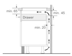
Measurements in mm
