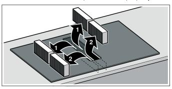
3. Insert two of the activated charcoal filters or acoustics filters into the left and right of the appliance and slide them forwards.
