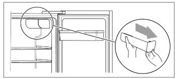
2. Open the refrigerator door to its maximum angle and remove the water filter cap by pulling it out slowly.
