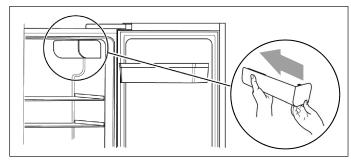
5. Reattach the filter cover by gently sliding it on.
