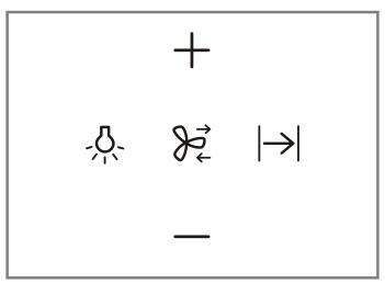
Increase fan setting / intensive mode / switch on appliance Decrease fan setting / switch off appliance Ŋ. Lighting Intermittent mode Fan run-on
