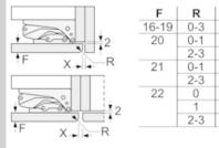
The gap dimensions recommended in the table must be adhered to in order to ensure that appliance doors do not collide with anything when they are opened, and to avoid causing damage to kitchen units.
