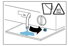
8. Firmly press on the sealing cap.
