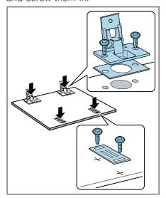
5. Screw on the counter plates for the magnetic catches.
