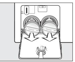
Remove the drain filters completely.
