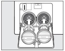
Replace the drain filters correctly (on the right and left) and tighten them securely. Risk of damage from leaking water.
