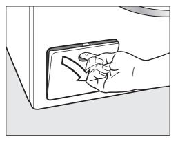
Open the drain pump access panel.
