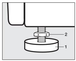
Using the open spanner supplied, turn counter nut 2 in a clockwise direction. Then turn counter nut 2 together with foot 1 to unscrew.
