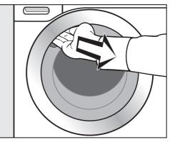
Reach under the recessed grip and pull the door open.
