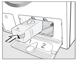
Push the UltraPhase 1 detergent cartridge into compartment 1 until it locks into position.
