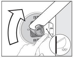
Push the cover out and turn the lefthand transit bar 90° using the open spanner supplied.
