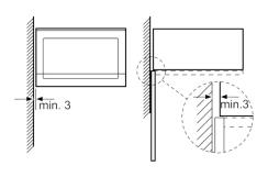
Measurements in mm
