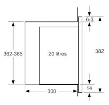
measurements in mm
