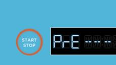
**6.** "PrE" and progress bars indicate unit is coming to steam temp. When unit switches to convection cooking, timer will start counting down.
