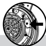
If the unit is not coming to pressure, check that the silicone ring is fully installed by pressing it into place all around the metal ring rack. Make sure the ring is completely clean and undamaged.
