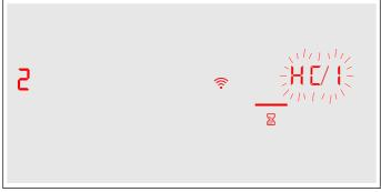
Use the "Home Connect" SSID and the "Home Connect" key to register the mobile device on the hob network.
