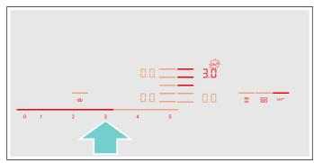
The function has now been activated. The temperature symbol flashes until the frying temperature is reached. A signal sounds and the temperature symbol goes out.
