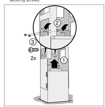
3. Hook in the retaining clip and screw tight.
