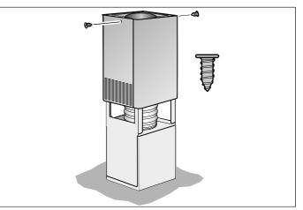
5. Insert both lower parts of the flue and push together.
