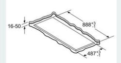
Never fit directly onto plasterboard or similar lightweight construction materials of the suspended ceiling. A suitable substructure is required that is securely fixed to the concrete ceiling.
