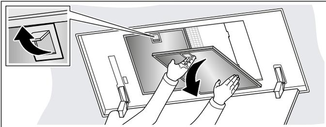
4. Take the metal grease filter out of the holder.
