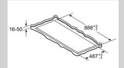
Never fit directly onto plasterboard or similar lightweight construction materials of the suspended ceiling. A suitable substructure is required that is securely fixed to the concrete ceiling.
