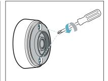
2. Open the closure of the temperature sensor. Remove the battery from the lower section of the housing and insert a new battery (pay attention to the correct orientation of the battery poles).
