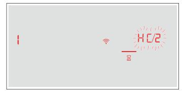
6. Start the app on the mobile device and follow the instructions for automatic network registration. The registration procedure has been completed once the  $\mathcal{G}$  value appears on the cooking position display.
