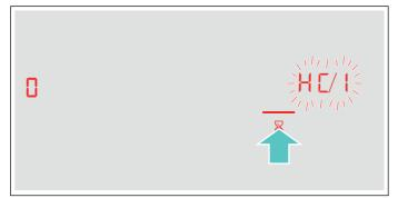
Set the 2 value in the control panel. In the control panel, 2 and the symbol 奈 flash.
