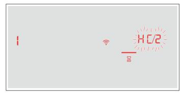
6. Start the app on the mobile device and follow the instructions for manual network registration. The registration procedure has been completed once the  $\mathcal{G}$  value appears on the cooking position display.
