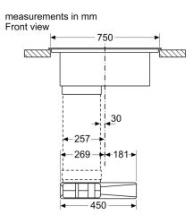
measurements in mm Front view – unit cut-out for unducted recirculation
