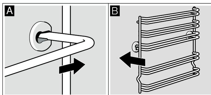
The rails fit both the left and right sides. Ensure that, as shown in figure B, levels 1 and 2 are below and levels 3, 4 and 5 are above.
