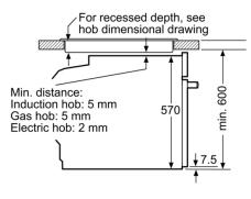
measurements in mm
