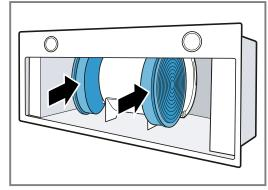
4. Install the grease filters.
