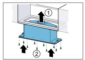
**2.** Tighten the fastening screws.
