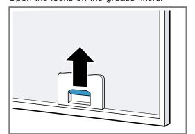
Remove the grease filters from the holders.To prevent grease from dripping, hold the grease filter horizontally.
