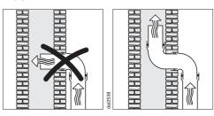
If the exhaust air is to be ducted into a flue, the ducting must be directed in the flow direction of the flue.
