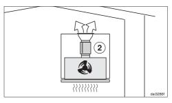
In recirculation mode, the silencer needs to be positioned between the exhaust vent and the exhaust grille ②. Check that there is sufficient space.
