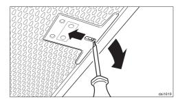
■ If the grease filter is inadvertently replaced the wrong way round, insert a small screwdriver blade into the slit to disengage the clip.
