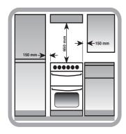
The height of the cooker can be adjusted by means of adjustable feet in the plinth (900mm - 915mm). Adjust the feet by tilting the cooker from the side. Then install the product into position. NOTE: This appliance must not be fitted on a platform. The cooker is
