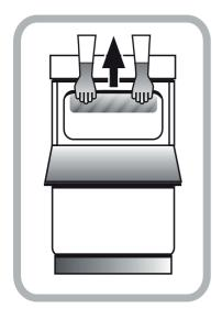
Before moving your cooker check that it is cool, and switch off at the cooker control unit.
