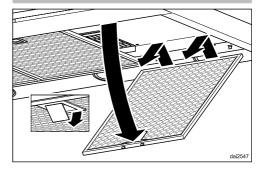
To take out a grease filter, release the locking clip on the filter, lower the filter approx. 45°, unhook it at the back and remove it.
