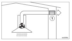
In extraction mode, the silencer not only reduces noise from the fan outside the house, but also sounds originating outside reaching the kitchen through the exhaust ducting (e.g. traffic noise). For this reason, the silencer must be positioned as close as possible to the ducting exit ①.
