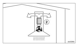
In recirculation mode, the silencer needs to be positioned between the exhaust socket and the directional unit (2). Check that there is sufficient space.
