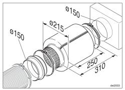
To reduce noise levels even further, a silencer (optional accessory) can be installed in the exhaust ducting.
