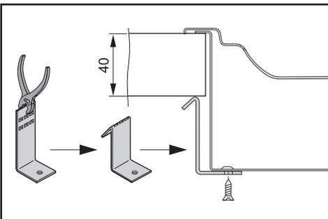
■ Secure the hob using the brackets supplied.
