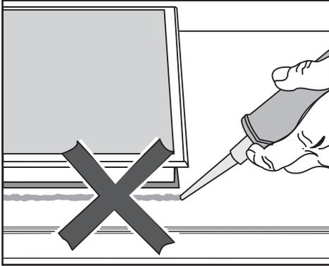
**⚠** Damage caused by incorrect installation.
