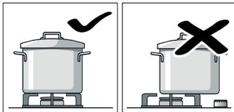
Always centre the pan over the burner, not to one side. Otherwise it could tip over. Do not place large pans on the burners near the control knobs. These may be damaged by the very high temperatures.
