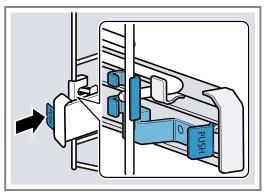
2. Keep the **PUSH** tab pushed back ① and swing the rail outwards ②.
