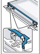
12. Attach the door cover ① and use a screw to secure it on the left- and right-hand sides 2.
