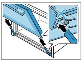
2. Using both hands, press down on the left and right of the door cover from above to check whether the appliance has been pushed in as far as it will go.
