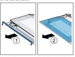
9. Loosen the screw on the left- and right-hand spacers a 1 and remove both spacers 2.
