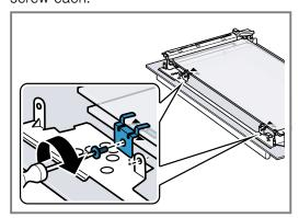
Slide the inner pane in. In doing so, ensure that the inner pane is in the retainer a.
