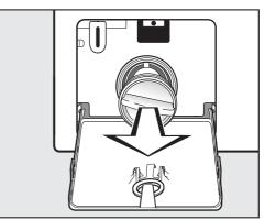
Remove the drain filter completely.
