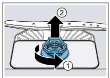
Pull down the micro filter to remove.
