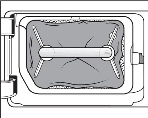
The edges of the plinth filter do not sit properly and the plinth filter is out of shape. Fluff will blow into the heat exchanger unfiltered through edges that do not sit properly. This will, in time, cause a blockage in the heat exchanger.
