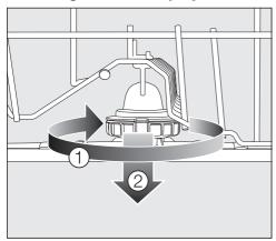
■ Rotate the screw thread of the middle spray arm clockwise ① and remove the spray arm ②.
