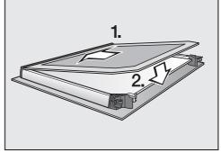
Push the inner pane with the matt printed side facing downwards into the plastic strip and place it between the retainers.
