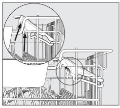
Pull the cup rack upwards and click it into the desired position (see arrow).
