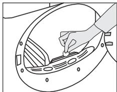
There are dampness sensors in the dryer that detect whether the laundry is dry or not. To clean the sensors:
