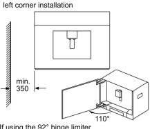
If using the 92° hinge limiter (spare part no. 00636455), the minimum distance to the wall is only 100 mm. measurements in mm
