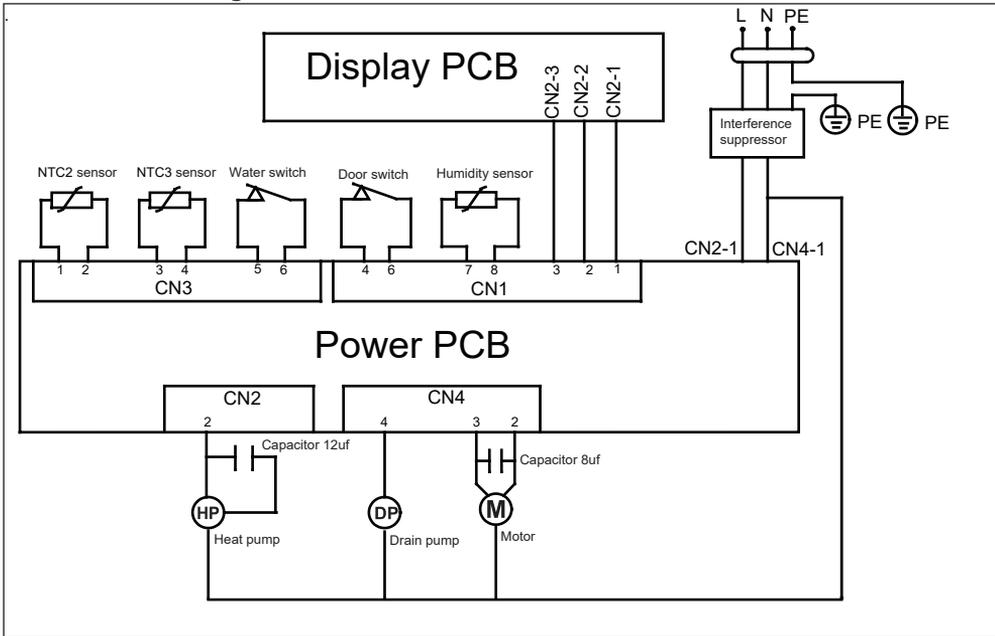
Electric circuit diagram HD80-A3959/HD90-A3959/HD90-A3959S:
