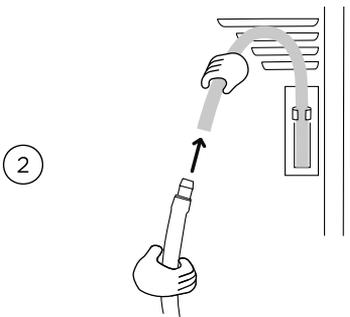
Uncoil the drain hose (included with your dryer) and connect it to the black hose.
