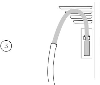
Place the other end of the drain hose into a tub or standpipe.
