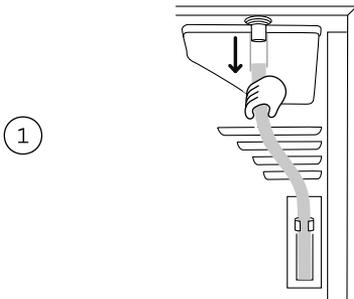
Remove the black hose from the connection at the back of the dryer.
