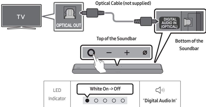
1. With the TV and Soundbar turned off, connect the **DIGITAL AUDIO IN (OPTICAL)** port on the Soundbar and the **OPTICAL** output port on the TV with the optical cable (not supplied), as shown in the figure.
