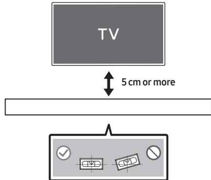
2. Align the **Wall Mount Guide's Centre Line** with the centre of your TV (if you are mounting the Soundbar below your TV), and then fix the **Wall Mount Guide** to the wall using tape.
