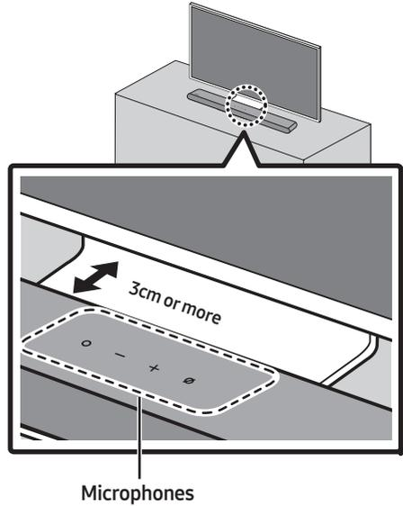
Align the centre of the Soundbar to the centre of the TV as illustrated in the image. At this time, place the Soundbar at least 3cm away from the TV so that there is no interference with voice recognition.
