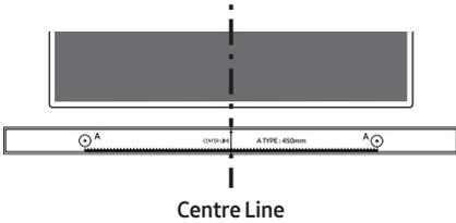
3. Use a pen to mark the positions of the holes and remove the **Wall Mount Guide**.
