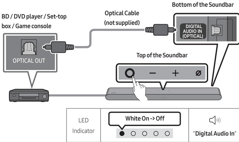
1. With the external device and Soundbar turned off, connect the **DIGITAL AUDIO IN (OPTICAL)** port on the Soundbar and the **OPTICAL** output port on the external device with the optical cable (not supplied), as shown in the figure.
