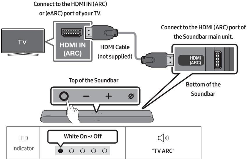
1. With the Soundbar and TV turned off, connect the HDMI cable (not supplied) as shown in the figure.
