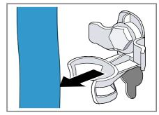
2 Unscrew ① and remove ② all of the screws for the 4 transit bolts using a WAF 13 wrench.
