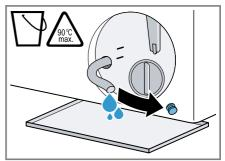
8. Firmly press on the sealing cap.
