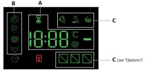
The duration of the available wash cycles and the remaining time of a running cycle appear in section A; if the Delayed Start option has been set, the countdown to the start of the selected cycle will appear. Pressing the corresponding button allows for viewing the maximum spin speed and temperature values attained by the machine during the set wash cycle, or the values selected most recently, if these are compatible with the set wash cycle.
