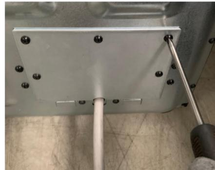
Assemble cover and tighten screws.
