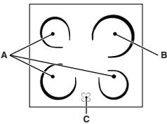
A. The cooking zone with radiant heating elements.
