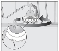
■ Replace the middle spray arm and turn the screw thread anticlockwise until it engages. Make sure that the recesses in the lock line up.
