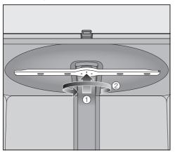
■ Push the upper spray arm upwards ① to engage the inner ratchet. Then unscrew the spray arm by rotating the screw thread anti-clockwise ②.
