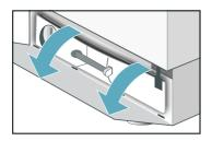
3. Take the drain hose out of the retainer.
