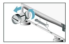
5. Replace the pump cover and screw firmly in place. Place the kick panel in the 4 clip-in slots and secure to the housing using the lock pins.
