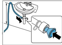
Secure the connection point with a (12-22 mm) hose clamp. Secure the water outlet hose with a hose guide at a height of at least 80 cm and no more than 100 cm.
