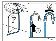
Push the water drain hose fully through the elbow → Page 12 and secure it using fixing material. Secure the elbow at a height of no more than 100 cm.
