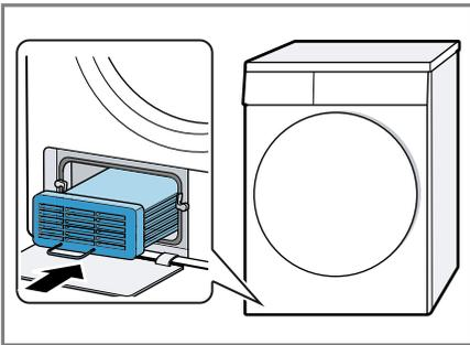
Ensure that the heat exchanger is inserted with its handle pointing downwards.
