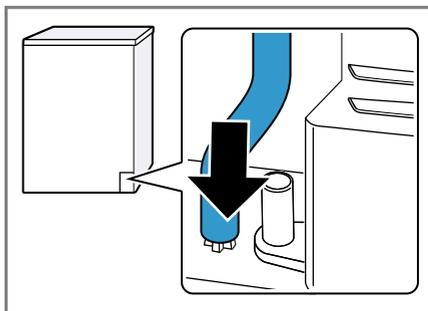
3. Push the water drain hose as far as it will go into the connecting piece.
