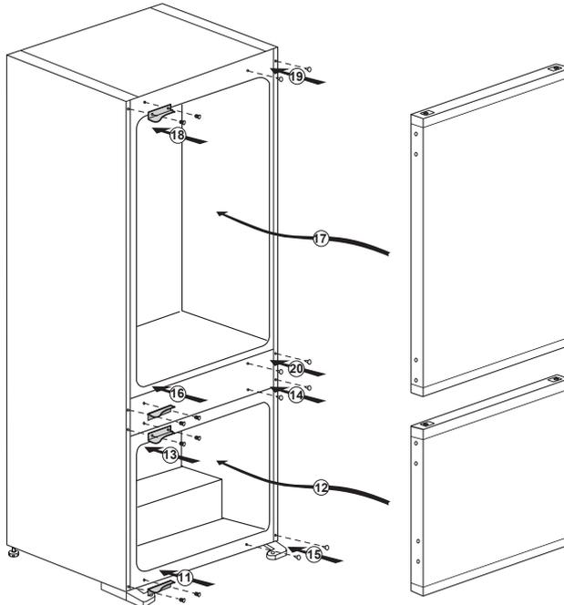
Refit plastic plugs (7, 8, 9 & 10) into the screw holes on the right hand side (14, 15, 19 & 20).
