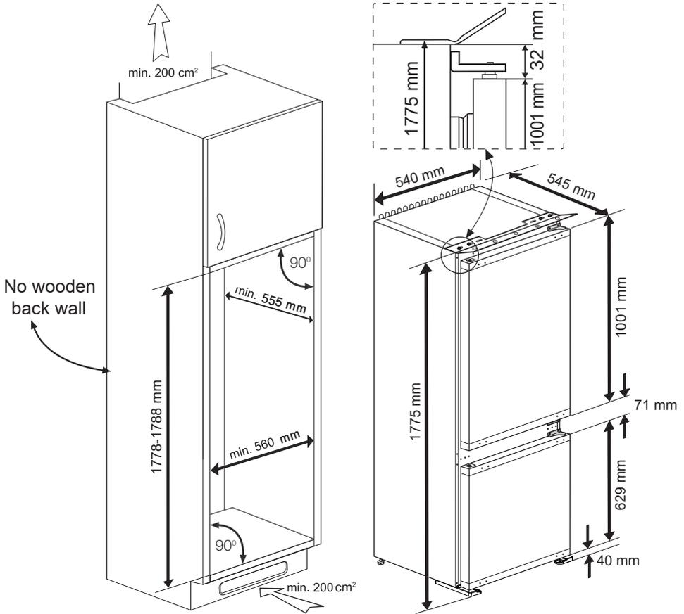
The back wall of the wooden cabinet must be left open completely to kitchen wall in order to allow sufficient air circulation to cool down the condenser unit for energy efficiency.
