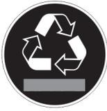
This or a similar sticker may be located on the rear of the appliance. This sticker indicates that there are vacuum insulation panels (VIP) or perlite panels in the door and/or housing. This advice is only relevant to recycling. Do not remove the sticker.
