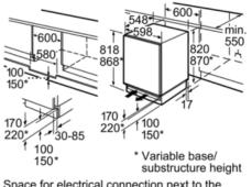
Space for electrical connection next to the appliance on the left or right-hand side. Ventilation space in the base.
