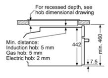
measurements in mm
