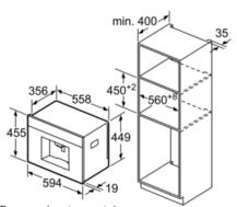
Bean and water containers are removed from the front. Recommended installation height 95-145 cm. measurements in mm
