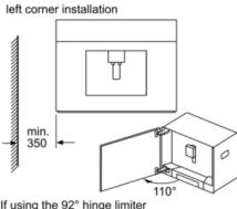
If using the 92° hinge limiter (spare part no. 00636455), the minimum distance to the wall is only 100 mm. measurements in mm
