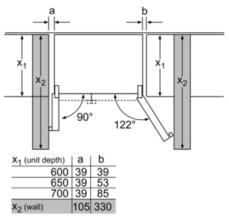
measurements in mm
