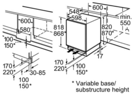
Space for electrical connection next to the appliance on the left or right-hand side.
